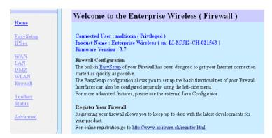
The Easy Setup window (below) allows for fast configuration of your MultiCom Firewall. After reading the warning click the "Next" button to start configuring the WAN interface.
