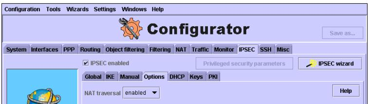
When enabled, the MultiCom Firewall allows IPSec clients behind a NAT device to build an IPSec connection that is encapsulated in UDP packets. There are some minimum requirements to use NAT traversal.
