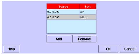
By clicking ADD the default suggests allowing access from anywhere in the Internet just to the WAN/PPP interface. This connection is secured by HTTPS and the incoming user still needs to authenticate with a valid username and password before they will have access to the MultiCom Firewall.
