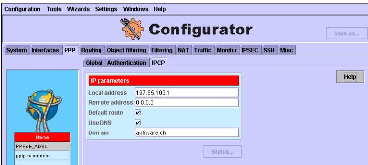
If you are using PPPoE or PPTP and your Internet Provider has given you a permanent IP address you can configure it on this screen. This will configure your MultiCom Firewall to always ask for the same IP address when it authenticates (your ISP must support this.)
