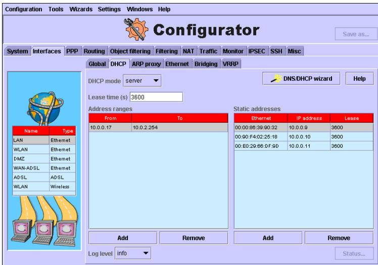
The DHCP Server of the MultiCom Firewall can either randomly assign IP Addresses within a preselected range or static entries can be given out based on the MAC Address of different Ethernet devices on the network.
