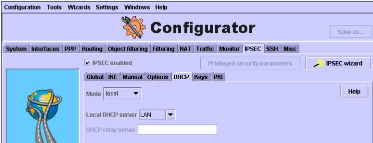
This feature is activated in the IPsec DHCP panel. A local interface with an already activated DHCP server or a remote DHCP server (identified with an IP address in the Relay field). Optionally these IPsec clients can appear to be on the local LAN by additionally using ARP Proxy.
