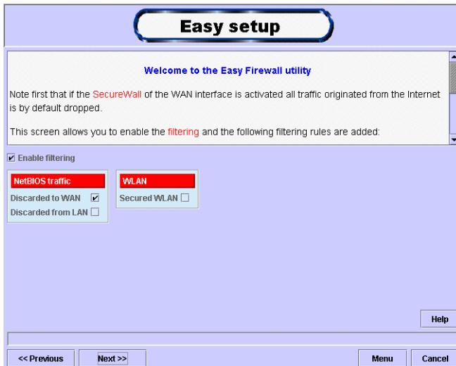
When this panel is disabled, the filtering system does not perform any traffic control. However if the SecureWall is active on the WAN interface it does act as a firewall (with all traffic coming from the WAN being dropped unless it is in response to a demand from the LAN.)
