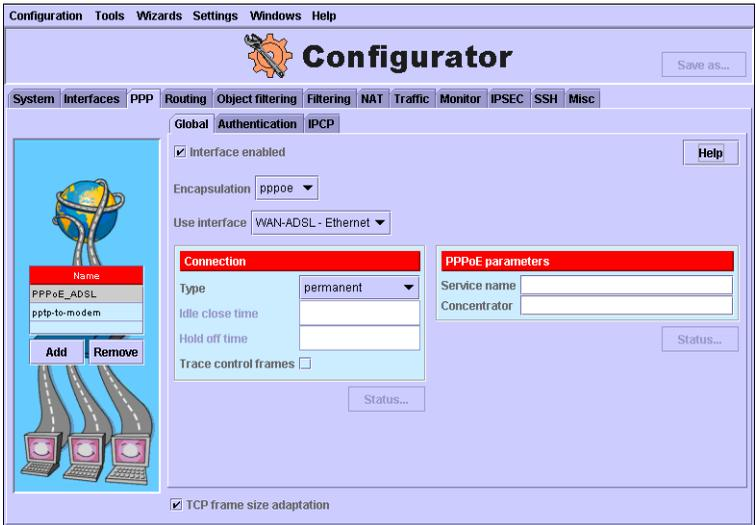
While it is possible to assign PPPoE connections to one or more physical interfaces of the MultiCom Firewall, each PPPoE connection must be enabled to be active. Disabled interfaces are stored in the configuration file but are inactive.
