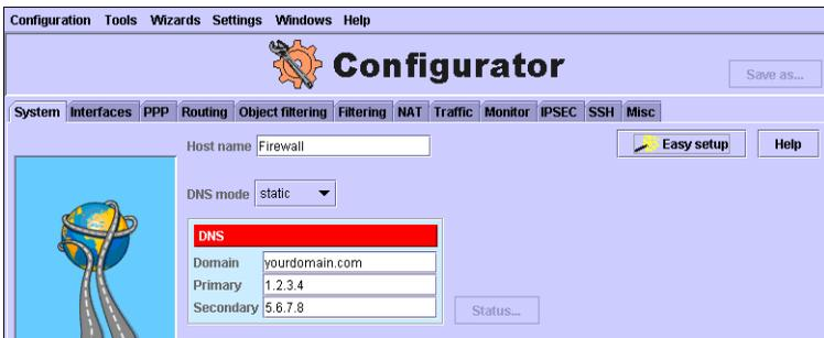
Dynamic configuration of Global DNS implies that information DNS information will be received through a protocol such as DHCP, PPPoE, or PPTP. For DHCP, received information (from the WAN interface's DHCP client for instance) is used by the proxy DNS or the DHCP server as in the case of a static configuration. For PPPoE, the problem becomes more complex. Because multiple PPPoE sites can be active simultaneously, it is possible to receive IP addresses for multiple DNS servers.
