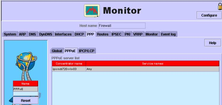
This PPPoE Server window displays the available PPPoE WAN Access concentrators and services that are available on the network attached to the MultiCom Firewall interface that is configured as a PPPoE interface. If no Concentrator is shown there is none available to give an IP configuration. If this is the case
