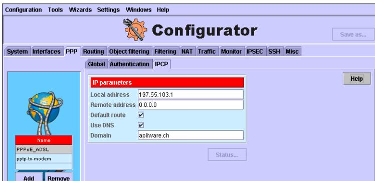
The DNS info received by the PPPoE sites can also change as it is given during the authentication process. It is not obligatory to assign a PPP connection a Domain Name. If no domain name is given and the Use DNS option is selected
