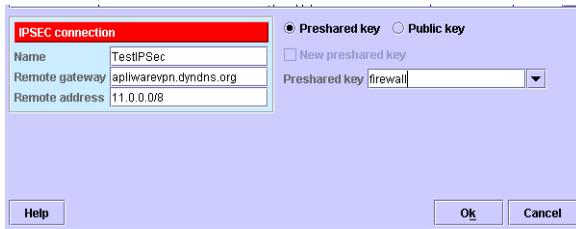
The Wizard will add a new IPsec connection with the chosen name to the configuration of the MultiCom Firewall. Additionally it will add NAT SecureWall rules to allow incoming IKE (UDP 500) and ESP traffic. Finally it will enable IPsec. Data traffic over the Internet between the 2 MultiCom Firewalls will be encrypted and traffic from the LAN to the Internet will not be encrypted.
