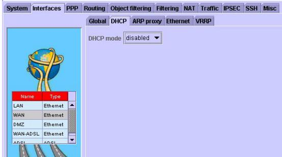
To set your computer to use static addressing (meaning each computer will manually be configured with all of the necessary information) you will need to set the LAN interface DHCP Mode to be disabled. You will also have to turn off the DHCP mode for the LAN interface. Finally, be sure that you have identified an IP address and subnet mask for the LAN interface.
