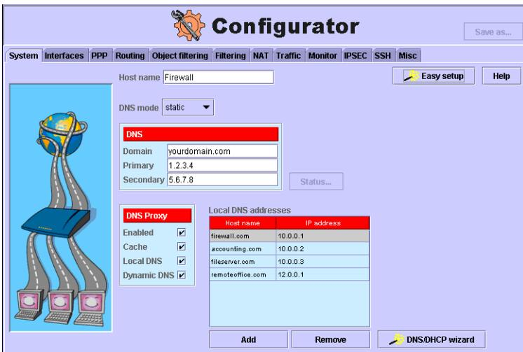
When the proxy DNS is activated on the System panel of the Configurator, the DHCP server sends its clients the IP address of the interface on which the DHCP server is configured as the IP address for DNS. This global DNS is not associated with a particular Domain Name as can occur with PPPoE sites.
