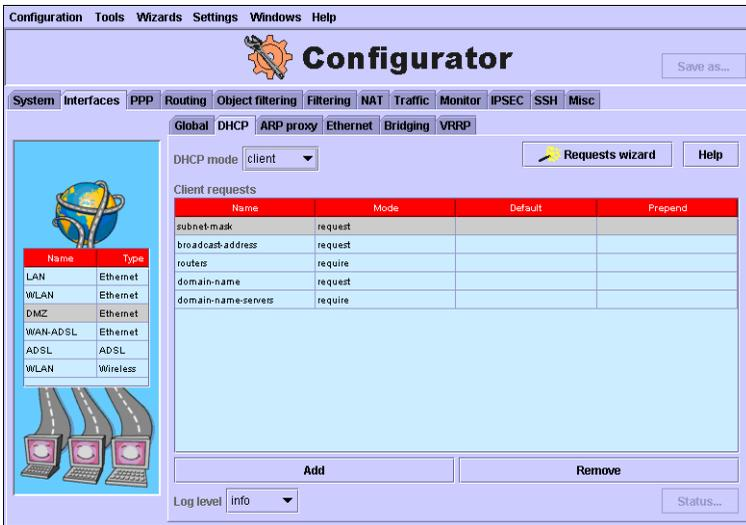
You have 3 different ways for preparing your firewall to interact with your network. Either it will act as a DHCP server and automatically give all of the necessary setup information to any computer plugged in to your network, you can configure the use of a remote DHCP server using DHCP relay, or you can choose the all manual route where every network device must manually be configured with the necessary settings to reach the firewall.
