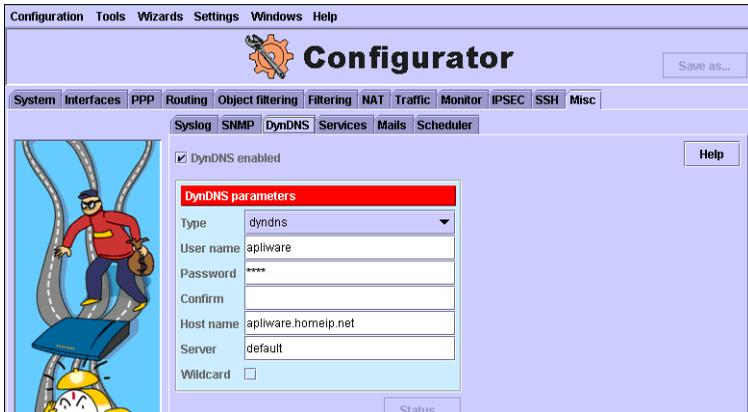
This is useful when the MultiCom Firewall does not have a fixed IP address but the user still wants to have a name on the Internet that the device can be found. When this service is configured the MultiCom Firewall will update the chosen dynamic DNS server with the current IP address of the WAN interface whenever it is changed.
