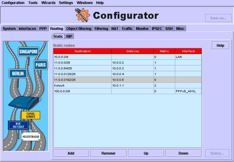
The screenshot shows the 'Configurator' application window. The 'Routing' tab is active, and the 'Static' sub-tab is selected. A diagram on the left illustrates a network topology with nodes labeled SINGAPORE, PARIS, BERLIN, CANAL STREET, RUE DU CHAT, and NEUSTRASSE. The main area displays a table of static routes:
