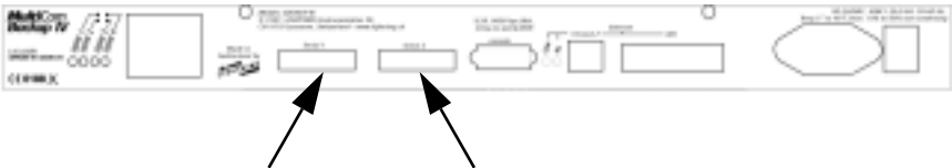
Figure 8 Serial port connectors
